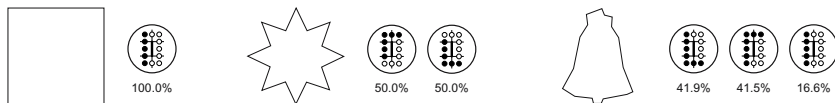
Fig. 3. Three simple scope histograms and their respective polygons. Left: The square's histogram contains only one entry, since all of its line segments have the same scope relation. Centre: Due to the polygon's regularity, the star's histogram consists of two entries with equal frequency. Right: The bell's scope histogram contains three entries.
