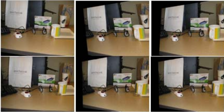
Fig. 4. Left column: original pair. Center column: rectified results based on Hartley's method. Right column: results of the proposed method.
